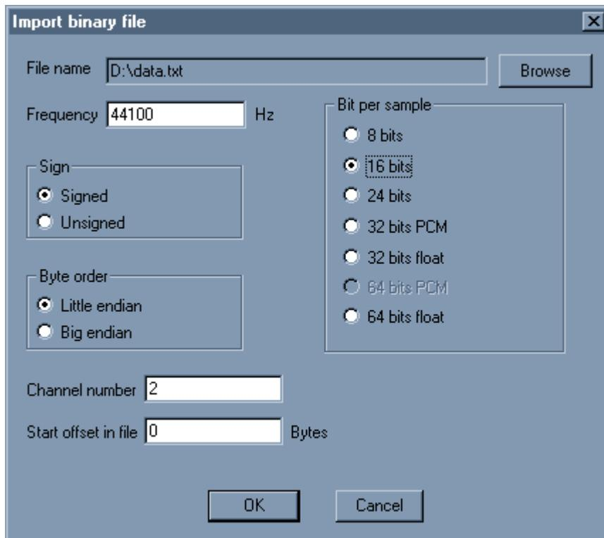
You can import any file, choose the settings for samplerate, bitdepth, sign, channel number and byte order. You can also select an offset to skip the first n bytes of the file.
