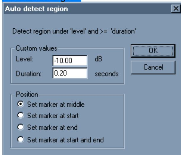
Insert markers automatically, based on time and amplitude threshold set by user. Can be useful to delimit regions separated by silence.
