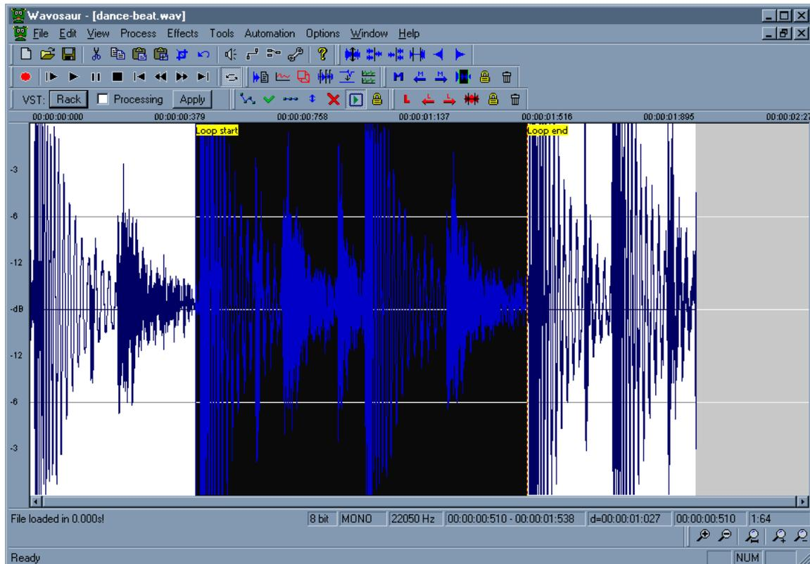
To insert loop points in your file, press the "L" key or go in menu Tools → Loop → Create loop points.
