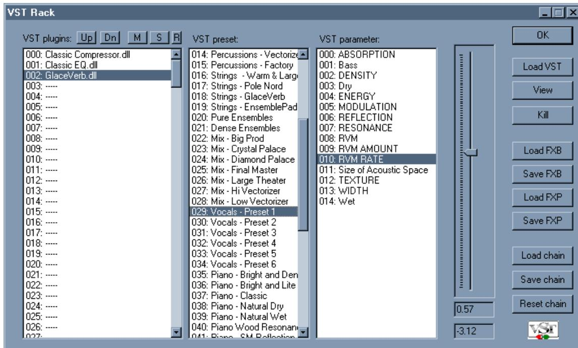
To chain the VST effects, select a slot and load a VST effect into it, the signal flow is as you expect : from the slot 000 to the last occupied slot.
