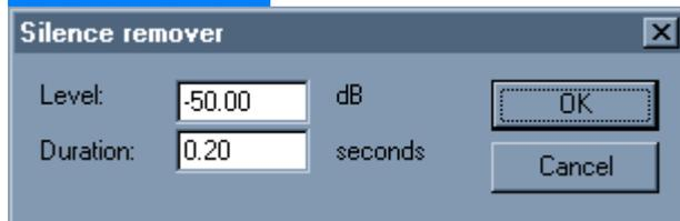
Automatically removes the silence in a file. "silence" can be defined by user, by setting threshold for minimum time and minimum amplitude.
